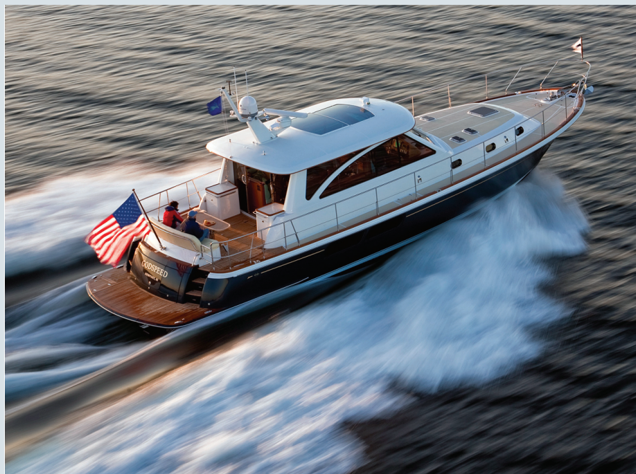
This Hunt 52 features a deep-vee hull with steep entry, bow flare and efficient chines.
