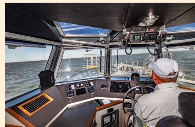
Foster heads for the sea buoy, off Cameron, La. The pilot boat's wheelhouse provides operators with easy-to-reach controls and impressive visibility. The foredeck, right, has port and starboard boarding platforms and a Harken rail and trolley system for increased pilot safety.
