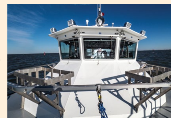
Foster heads for the sea buoy, off Cameron, La. The pilot boat's wheelhouse provides operators with easy-to-reach controls and impressive visibility. The foredeck, right, has port and starboard boarding platforms and a Harken rail and trolley system for increased pilot safety.
